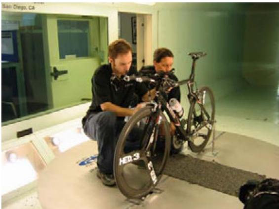
Kestrel engineers prepare for another test run (Kestrel/San Diego Low Speed Wind Tunnel)
